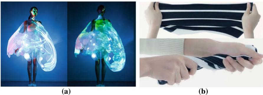
Fig. 12. Buble Emotion Sensing Dress. Design group at Royal Philips Electronics, Netherlands. 2007 [19]; Fabric Strain Sensor, AdvanPro. Hong Kong [20]
