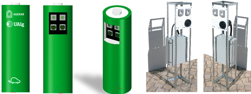
Fig. 5. 3D modeling of the EVSE (left and central images) and its current internal implementation (right side images).
