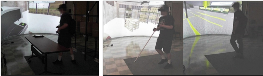
Fig. 5. Left: Picture of the real walking locomotion technique in the VR4VR system. The user walks inside the tracked area in the shelving module. Right: Pictures of the walk-in-place locomotion technique in the VR4VR system. The user navigates in the virtual world by walking in place in the real world. (left) Cleaning module, (right) environmental awareness module.
