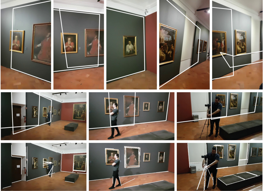
Fig. 6. Top row, examples of different vertical matching outcomes. Middle row, initial results of matching while the view is obstructed by persons. Bottom row, examples of the Hough Transform [26] applied to different frames.
