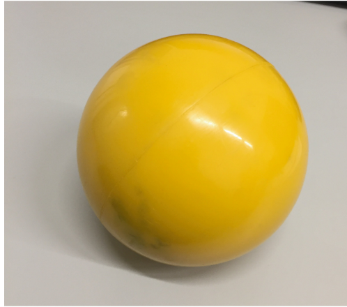
Fig. 5. Ball used at Real task. The weight was 220 g and diameter was 80 mm.
