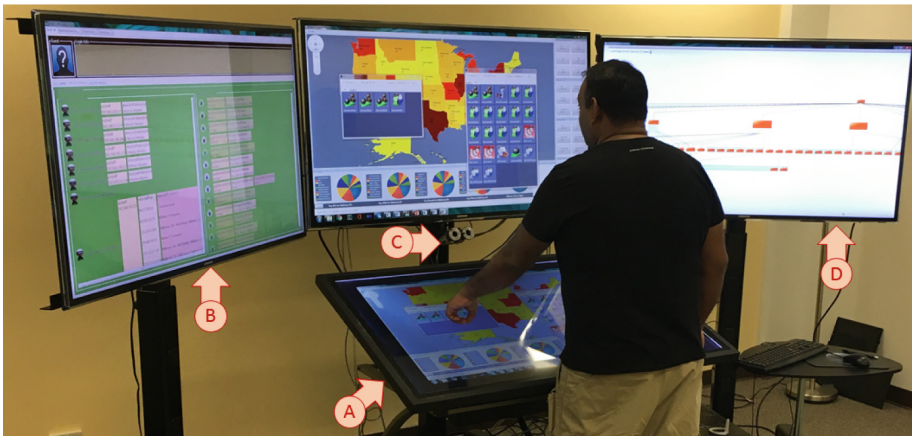
Fig. 1. bRIGHT workstation and its main components: (a) multi-touch surface, (b) backend server, (C) gaze tracker, (D) Contextual Model
