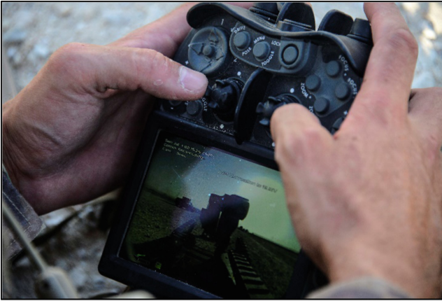
Fig. 1. Interface for teleoperation of a PacBot 310 robot, [5]
