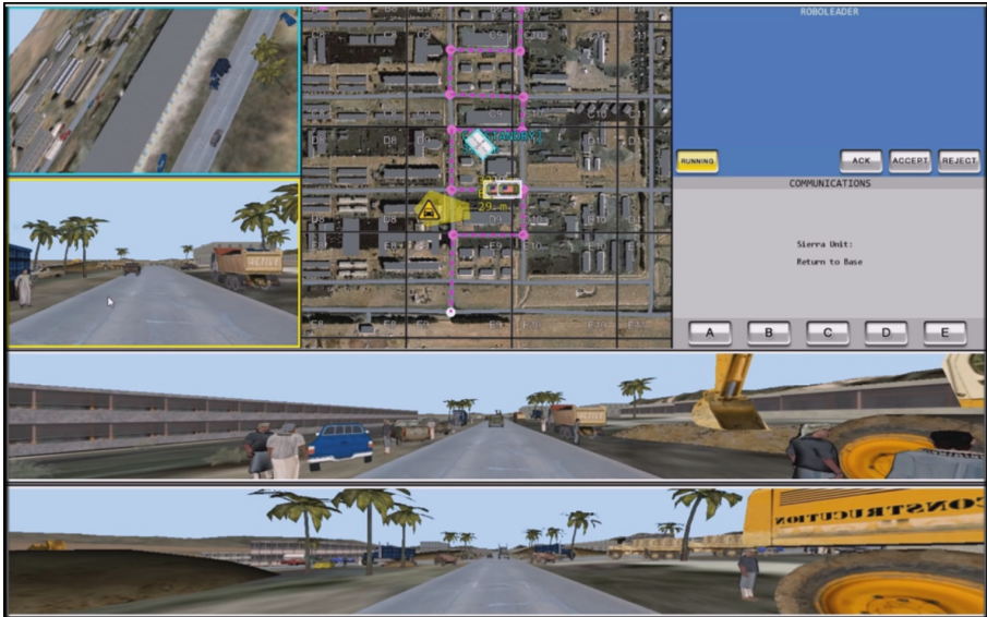
Fig. 3. MIX Testbed Operator Control Unit (OCU) simulation. OCU includes video feeds from multiple robots (i.e. air, ground) and a 360 degree indirect vision display, map for route/mission planning, and dialogs for interaction with automated agents and command, [26]. Users configure OCU layout, graphics, content, and scenario using XML.
