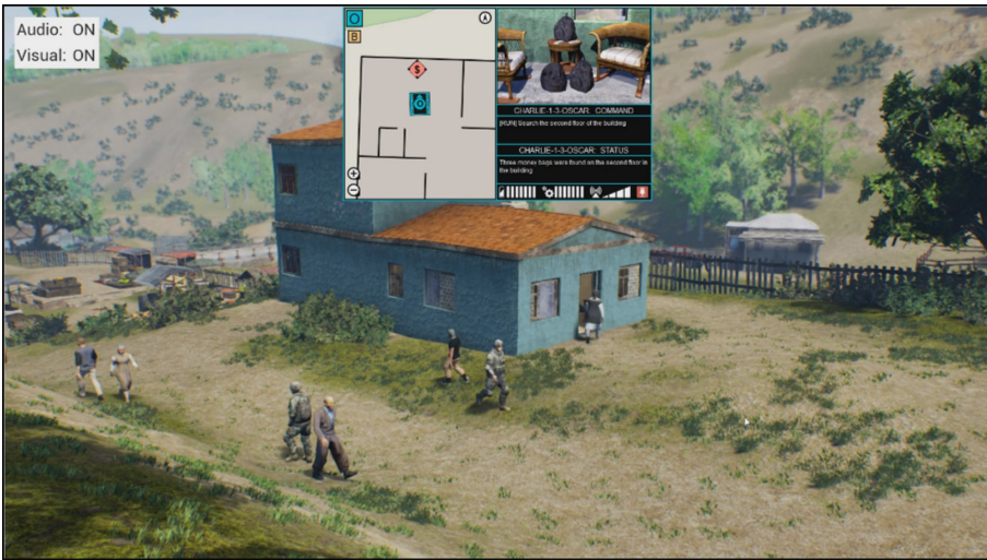
Fig. 4. VTB and MMI Simulation for dismounted human-robot teaming. VTB generates virtual world images, content, and simulated robot, with the MMI (overlaid top-middle) supporting interactions with the robot and other simulated communications and tasks. Characters moving in the environment support a signal detection task.
