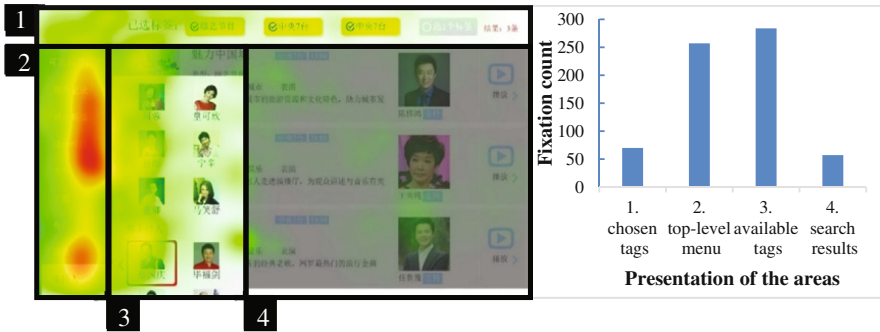
Fig. 3. Heatmap (left) and fixation count (right) of the mega menu. (Note that the numbers (1–4) represent the coding of the four areas in the black rectangular boxes.)
