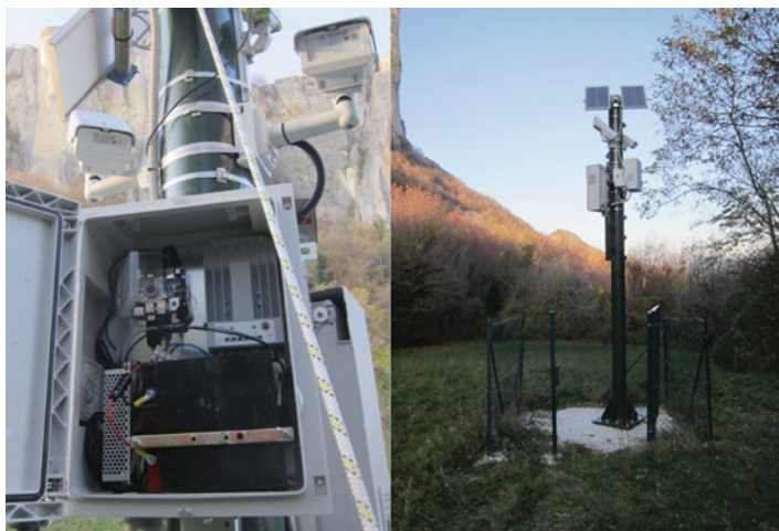
Fig. 13.1 Left: Beesper SmartBridge prototype. Right: Beesper SmartBridge prototype installed on a pole
