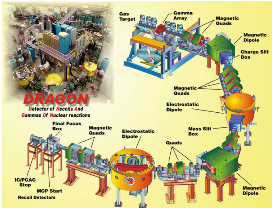
Fig. 9.2 The Dragon facility in Vancouver, Canada, is an example of nuclear experiment facilities, now aimed at experiments for astrophysically-relevant reactions: Radioactive isotopes can be selected and accelerated to form projectiles for such reactions of interest
