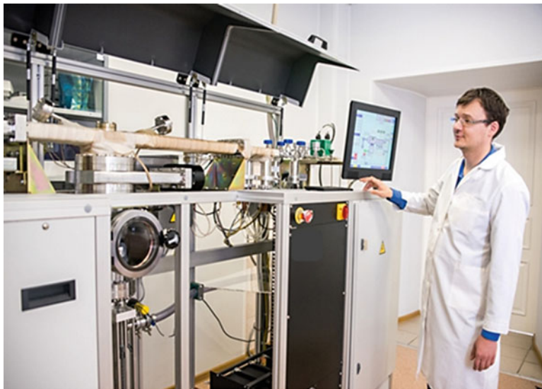
Fig. 4.2 Photograph of 2nd generation of molecular layer epitaxy setup
