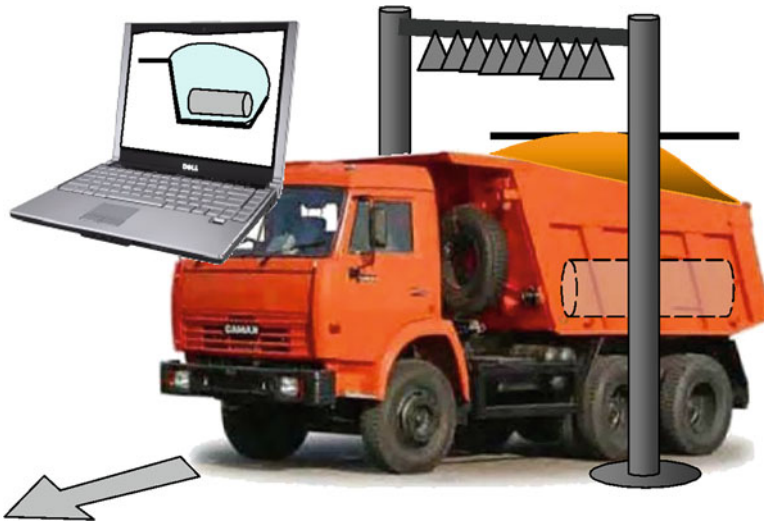
Fig. 8.23 Advanced system for detecting and visualizing hidden objects at ACPs
