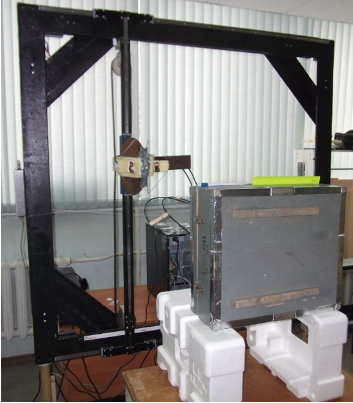
Fig. 8.17 UWB scanner and carrying box
