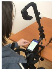
**Fig. 4.** Mobile eye tracking setup.
