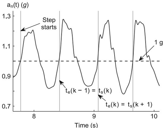
4. The step end  $t_e(k)$  is considered to be found when the next step starts or when a predefined time, considered as the maximum duration of one step, has passed after the start of the current step.
