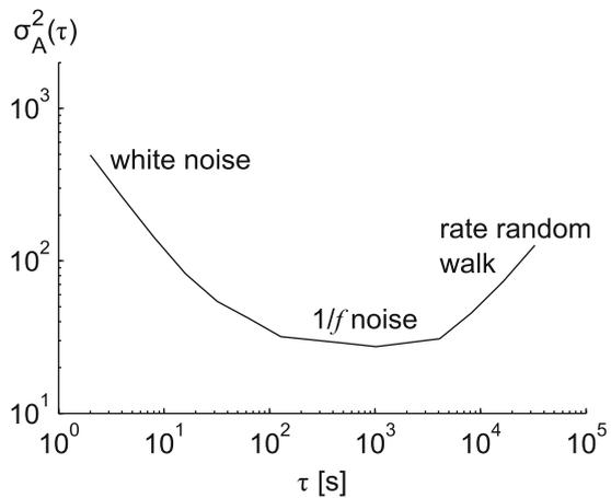
value of the descending white noise slope at  $\tau = 1$  s. The minimum value of the Allan variance between the white noise and rate random walk slopes corresponds to the square of the bias instability of the sensor; this value is directly related to the power of  $1/f$  noise [64].
