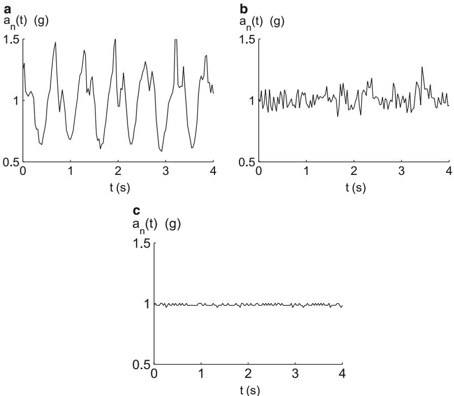
**Fig. 9** Norm of accelerometer output in different motion modes: (a) walking,  $\sigma = 0.24$  g; (b) driving,  $\sigma = 0.071$  g; (c) stationary,  $\sigma = 0.0084$  g
