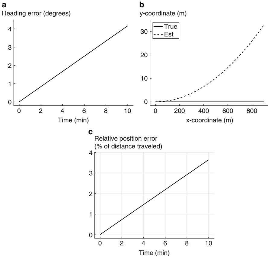
**Fig. 7** Effect of 25°/h gyro bias when the pedestrian is walking with constant speed along the positive  $x$ -axis: **(a)** heading error; **(b)** true and estimated coordinates; **(c)** relative position error
