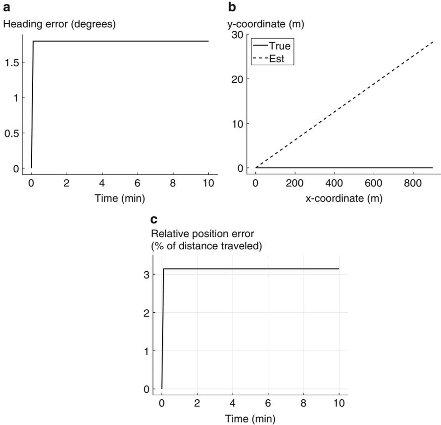
**Fig. 8** Effect of 1% gyro scale factor error when the pedestrian has made a 180° turn from  $-180^\circ$  and then walks with constant speed along positive  $x$ -axis: (a) heading error; (b) true and estimated coordinates; (c) relative position error
