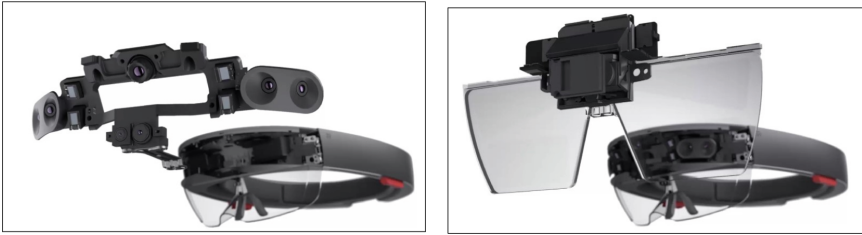
Fig. 4. HoloLens: sensor assembly (left) and display assembly (right), images taken from [17].
