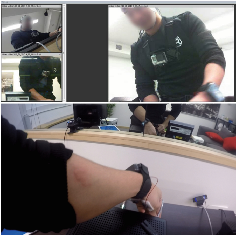
Fig. 2. Three cameras installed around the task area and a GoPro camera on the chest of the participant
