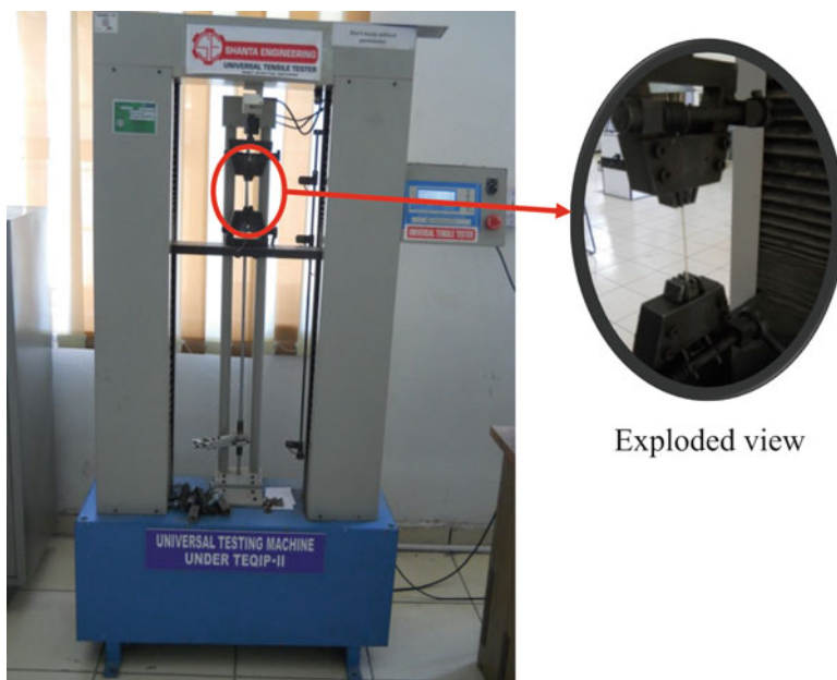
Fig. 11 Tensile test using Universal Testing Machine
