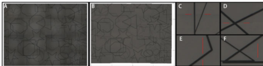
Fig. 6 Correcting results. (a) Before correcting. (b) After correcting and mosaic. (c–f) Zoom-in view of details in the joint area of two neighboring images. Red lines indicate the boundary of the images
