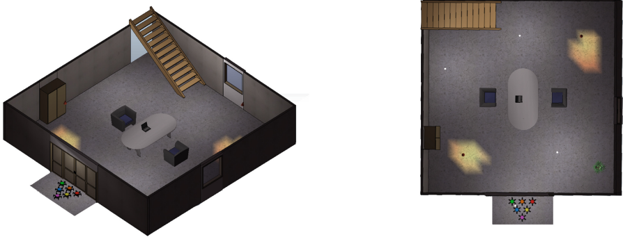
Fig. 2. Visual representation of the simulated setup yielding the results later discussed in the manuscript; (left) isometric view; (right) top-down view. The robot dynamics are provided by the VREP framework, whereas the NSGA-II routing approach has been implemented in Python and communicates with VREP via remote API functions.
