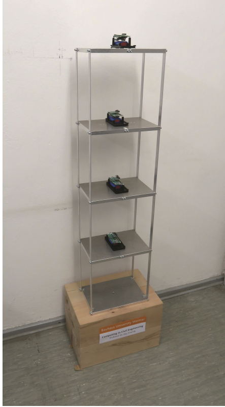
Fig. 7. Wireless SHM system installed on a laboratory test structure for validation.
