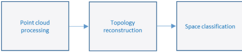
Fig. 1. Steps in space classification from point clouds.
