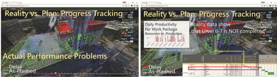
Fig. 11. Production and productivity rates are tracked per work package or trade to be transformed into actionable data.
