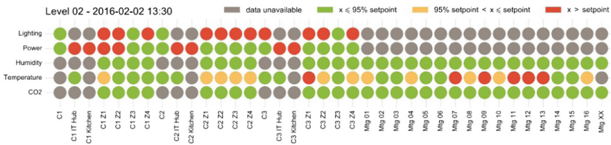
Fig. 14. Snapshot of the dashboard with interactive settings to override and adjust sensitivity settings for the indicators
