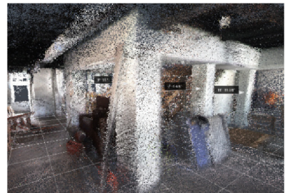
b. Mobile Lidar Based Point Cloud
