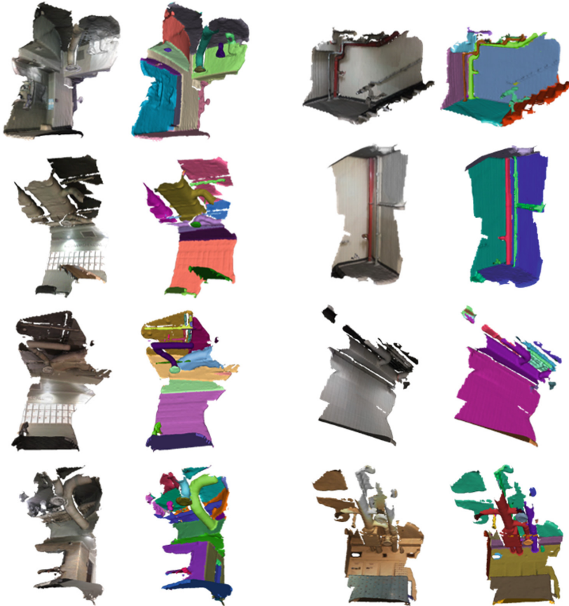
Fig. 8. Example annotated scans in 3DFacilities. Left: reconstructed surface mesh with original color texture. Right: each object instance shown with a different randomly assigned color. (Color figure online)
