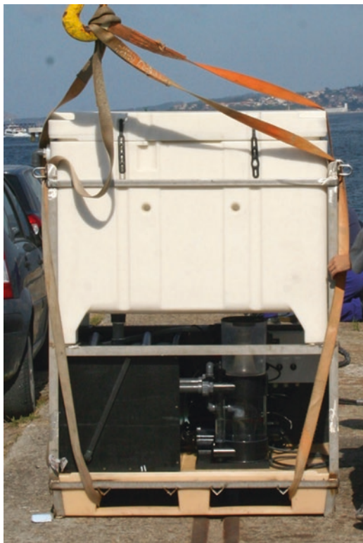
Fig. 38.1 The isothermal tank used by the Aquarium Finisterrae to keep deep-sea fauna alive at sea. The tank is located on the top of the so called “vital support” system which contains a skimmer and mechanical, chemical and biological filters (all of them placed in the black box). Behind the isothermal tank (not visible in the photograph) are located the ultraviolet unit as well as the chiller. (Photo: © A. Veiga)
