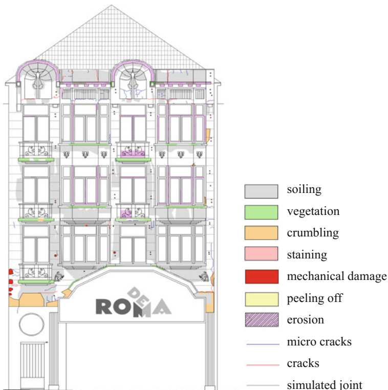
Fig. 5 Damage assessment of the north façade (Govaerts 2012)
