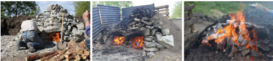
Fig. 8 Lime kiln during the first, second and third day. On the third day the flames started to become blue all over the top of the kiln, giving a signal that the lime was burned long enough
