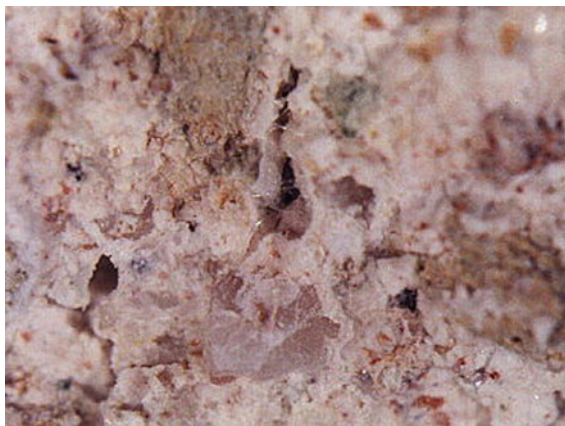
Fig. 1 Salt crystallization into the pores of a structural mortar from Galerius Palace (4th century AD)
