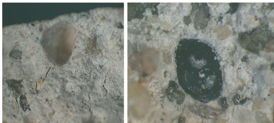
Fig. 3 Stereoscopic observation of salt crystallization into mortars
