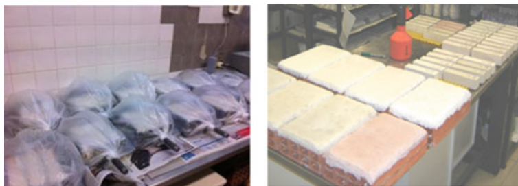
Fig. 2 Prismatic samples inside the moulds and conditioned in polyethylene bags; mortars on brick and prismatic samples at laboratory controlled conditions
