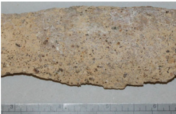
Fig. 5 M3 mortar with white crust on its outer surface
