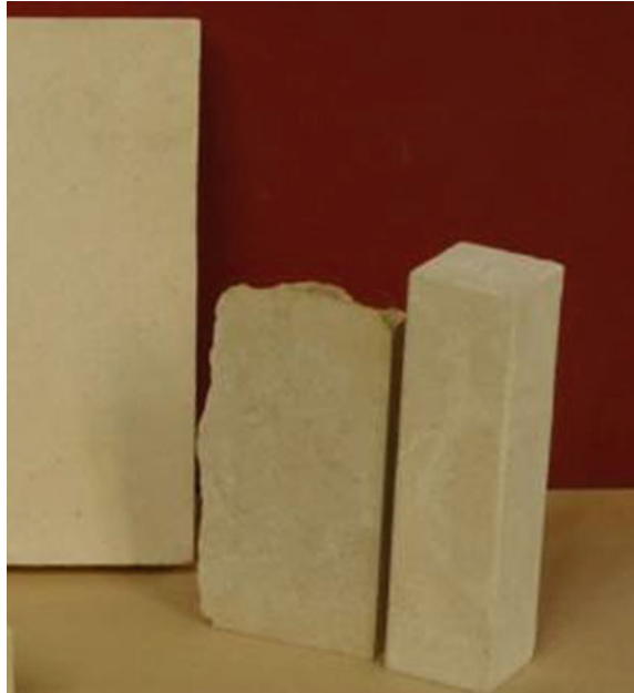
Fig. 4 Comparison between the original Tuffeau de Lincant in the middle and the mortar from the auto-formulation tool on the right
