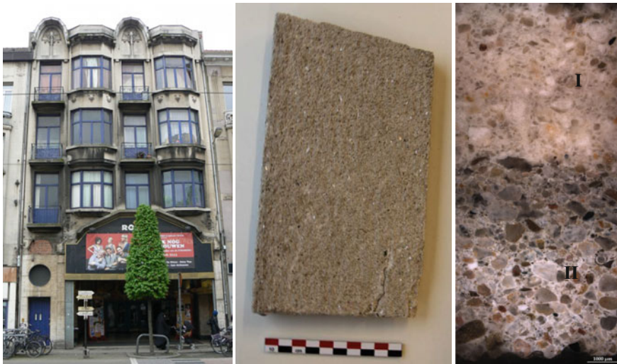
Fig. 1 Historic cinema “De Roma” (1928, north façade), Antwerp (Belgium): upper floors are finished with Terranova (Picture: Y. Govaerts) [left]; Terranova sample from the west façade of “De Roma” (Picture: L. Dekeyser) [middle]; Optical microscopic image of the layered structure of the historic sample: I. Top layer, II. Rendering layer (KIK-IRPA 2011) [right]
