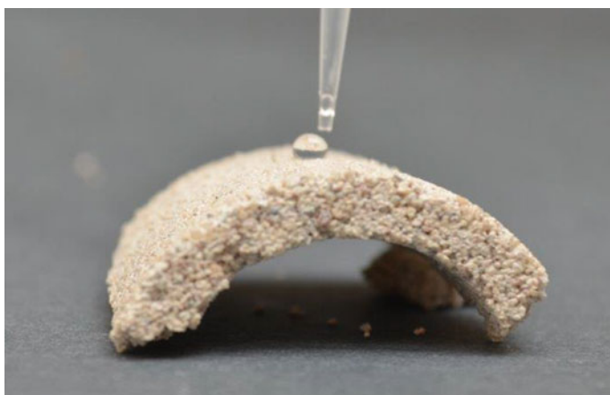
Fig. 5 Test of the water drop absorption rate
