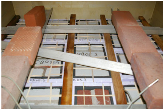
Fig. 5 The test specimens in the freeze-thaw container
