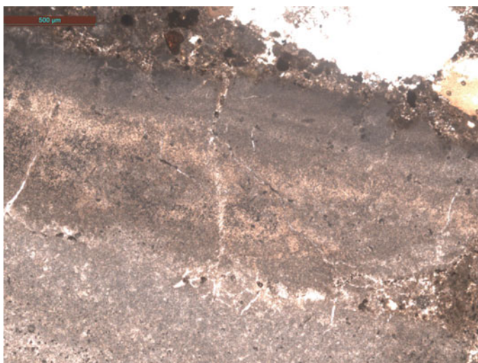
Fig. 4 Thin section of mortar from eastern cell displaying calcined and fractured shell with complete loss of internal microstructure. XPL. Scale bar 500 µm ( Photomicrograph M. Thacker )
