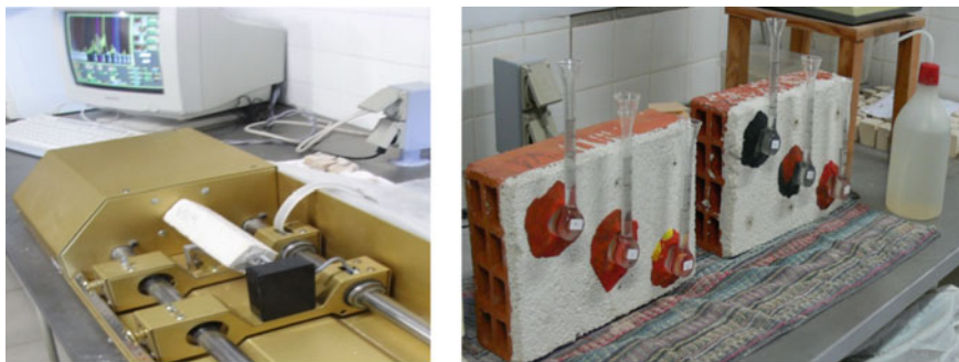
Fig. 3 Tests of dynamic modulus of elasticity and Karsten tubes
