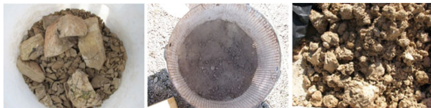
Fig. 10 Burned limestone from Marieby; dry-slaked Näsersjöberg lime in a special constructed steel basket; wet-slaked Marieby lime. The lime from Näsersjöberg is almost a bit purple-grey when it is slaked compared to lime from Marieby that is yellow-brown (Color figure online)
