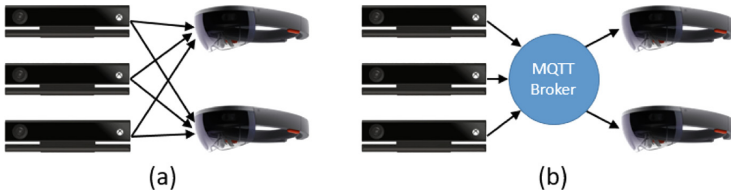
Fig. 5. Two alternative communication models: (a) UDP-based direct communication and (b) MQTT-based indirect communication.
