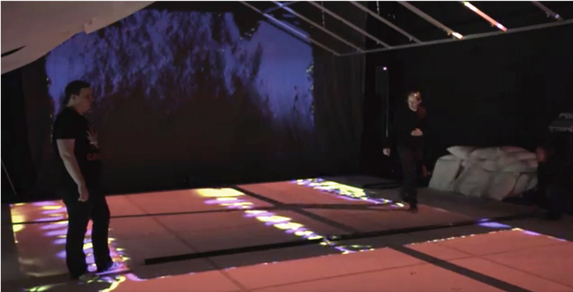
(b) Two researchers study changes to a simulated vortex sheet by narrowing a slit between two poles. The angle of air velocity is mapped to hue, with a constant external source of wind coming from upstage. Velocity magnitude orthogonal to the wind is sonified by averaging the velocity field over a coarse grid and spatializing the sound according to the grid cell centers.
