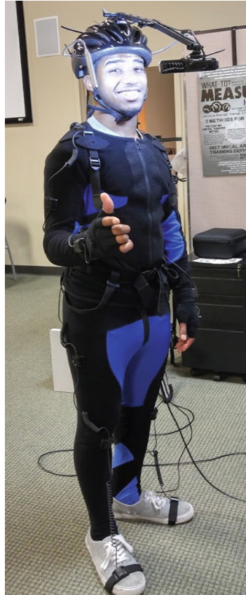
Fig. 2. Head-mounted prototype with sensors on motion capture suit
