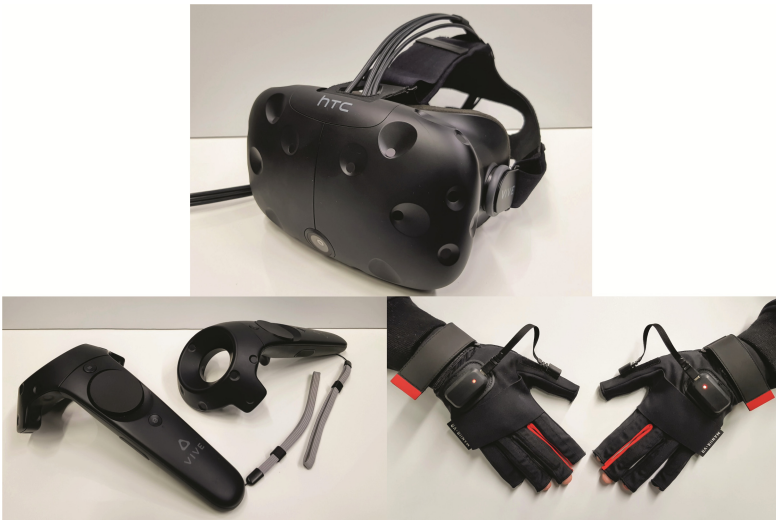
Fig. 2. VR set-up for the VLB implementation, top: HTC Vive HMD, left: Vive controllers, right: manusVR gloves.
