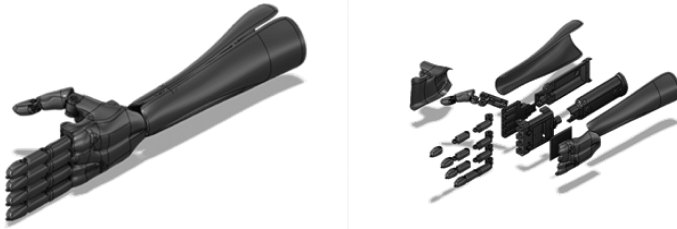
Fig. 2. Multi-gesture bionic hardware design on right with exploded view on left
