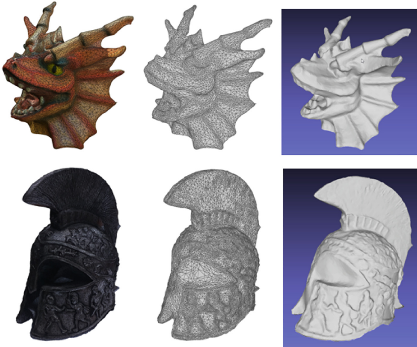
Fig. 5. Mesh surfaces with texture (left) and without texture (middle) in Autodesk ReCap, and model in STL format in Meshlab (right).
