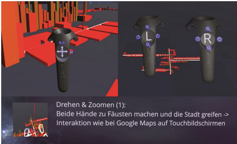
Fig. 7. Help system: top - help signs on the controller, bottom - explanations of an interaction possibility with video (Translation of the text: “Rotate & Scale (1): Make a fist with both hands and grab the city -> Interaction like with Google Maps used with touchscreen”).
