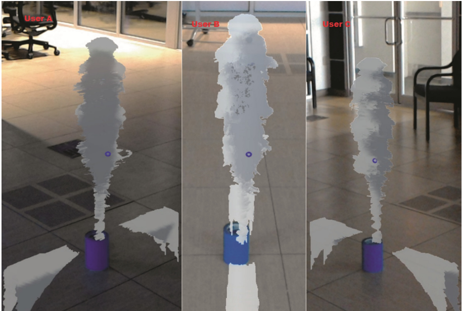
Fig. 3. Views from three Microsoft HoloLens showing the placement of 3D holographic object on top of a blue cylinder in the actual environment. From left to right, User A, User B, and User C respectively as viewed from their position as shown in Fig. 2. (Color figure online)
