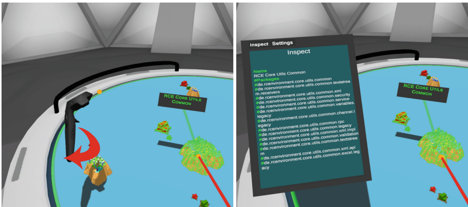
Fig. 7. To activate the VPDA, the underside of the controller is rotated into the users field of view, providing access to additional textual information and functionality.
