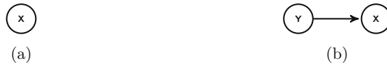
Fig. 5. Equivalent Markovian graphs associated to HCTBNs as introduced in Fig. 3: (a) \mathbf{Y} = \pi(X) = \emptyset ; (b) \mathbf{Y} = \pi(X) = \{Y\} .
