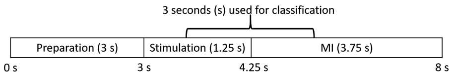
Fig. 1. Scheme of the MI capture session protocol. Notice that only three seconds of each trial were used in the classification process.
