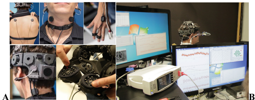
Fig. 1. RSS prototype sensor hardware and software. A: (top row, left to right) Trapezius muscle EMG and chest strap of ECG/respiration sensor; neck electrodes and throat microphone; GSR electrodes and pulse oximeter probe; (bottom row, left to right) ExG headset with additional sensor inputs; fNIR/EEG head set with coaxial EEG/fNIR sensor. B: AMI agent implementation for DACS utilizing multiple software agents to collect data from the RSS. It includes agents that manage experimental protocol administration and analysis algorithms for determination of ACS.
