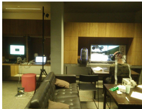
Fig. 2. Illustration of the experimental set-up with the participants playing the game in the virtual reality condition. The computer on the left provides the oddball task, whereas the laptop in the middle is used to record the EEG and the gaming computer with flat screen and the HTC Vive on the right display the game.
