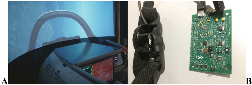
Fig. 7. A: DACS cockpit simulator example during ACS provoking event. During a standard-rate left turn, the pitch response to the control stick input reversed intermittently. This caused unpredictable aircraft behavior and pilot induced oscillation (PIO). B: left , Peltor throat microphone and, right , initial prototype low noise multistage amplifier and digitizer PCB.
