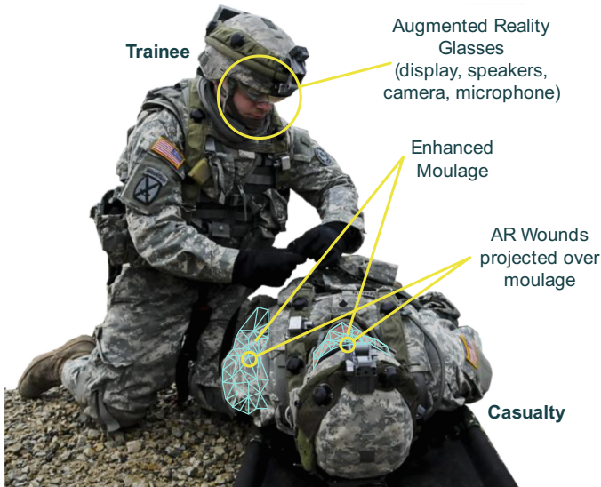
Fig. 2. Combat casualty care augmented reality intelligent training system (C3ARESYS) Concept (adapted from US Army photo).
