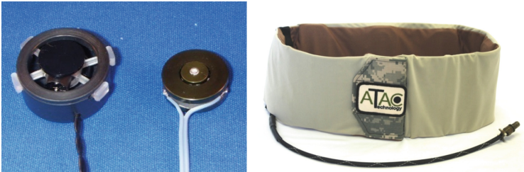
Fig. 1. EAI EMR and C-3 factor transducers (left to right), and 16-factor tactile belt
