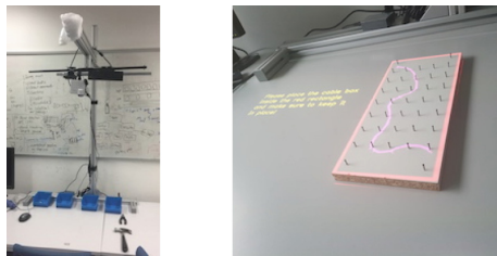
Fig. 2. Left: camera-projector setup with RGB-D camera. Right: step instructions are projected on the table.
