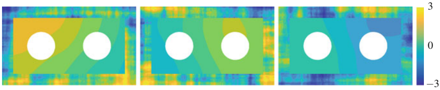
Fig. 3 Example realizations of the (zero-mean) Gaussian fields Z^{\text{int}} and Z^{\text{ext}} used in the heat exchanger problem. The insulator material has a lower correlation length and smoothness, and a higher variance. The associated conductivity is k = \exp(Z^{\text{int}} \cup Z^{\text{ext}}) . The number of terms used in the KL expansions for Z^{\text{int}} and Z^{\text{ext}} is 512 and 8 192, respectively
