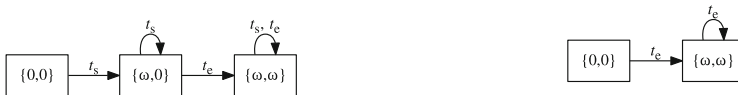
Fig. 5. Left: the BCG of the NS in Fig. 3 with t_1 and t_2 explicit. Right: the BCG of the NS in Fig. 3 with t_1 relevant and t_2 explicit. The firing vectors are omitted on the edges.
