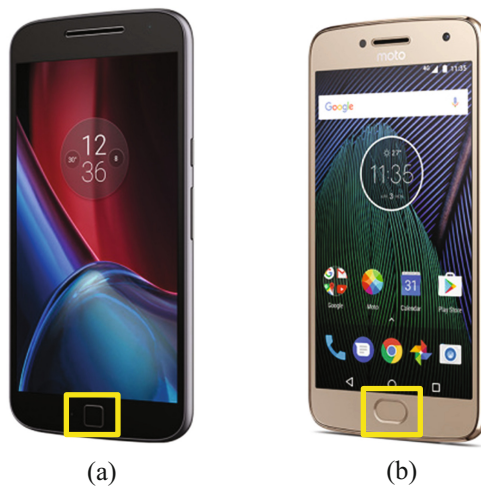
Fig. 1. (a) Moto G4 Plus and (b) Moto G5 Plus. Fingerprint sensor in both devices is highlighted.
