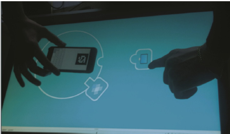
Fig. 2. Block-oriented programming with tangibles. Users are assigning digital properties and functionalities to a smartphone assembling blocks instead of by programming.
