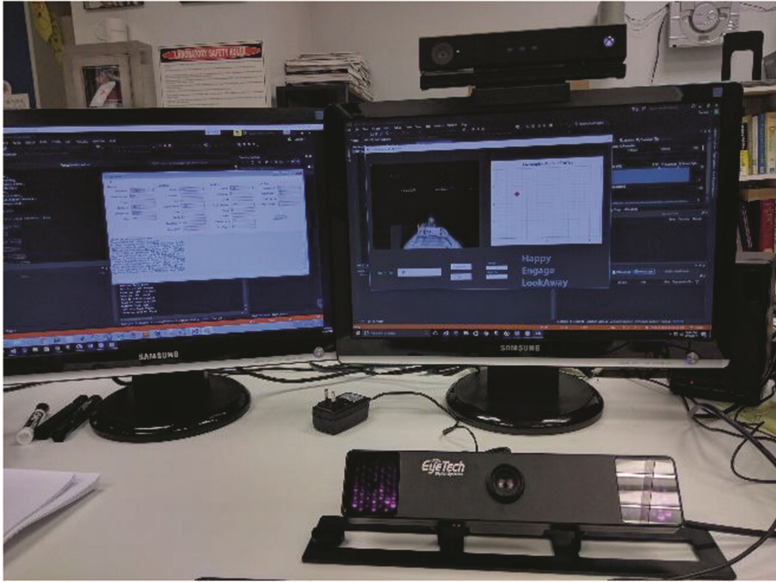
Fig. 4. Entire system including Kinect V2 (on top of the screen) and TM3 (in front of the computer).
