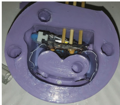
Fig. 5. Preparation for silicone casting
