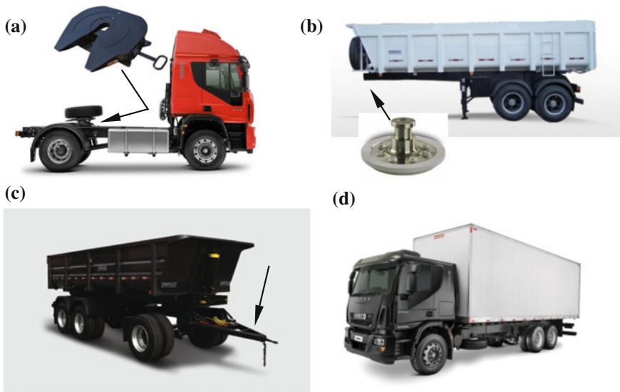
Fig. 1 a Fifth wheel and tractor truck [2, 3]; b kingpin and semi-trailer [2, 4]; c trailer unit with coupling device [5]; d box truck [3]
