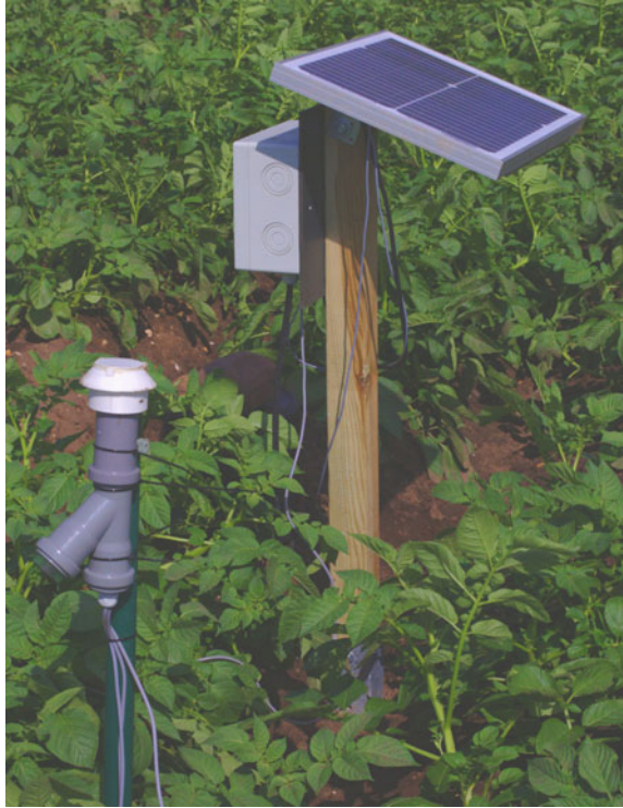
Fig. 17 Photo of a deployed node with several sensors attached
