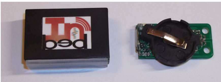
Fig. 22 Specialized InBED sensor node
