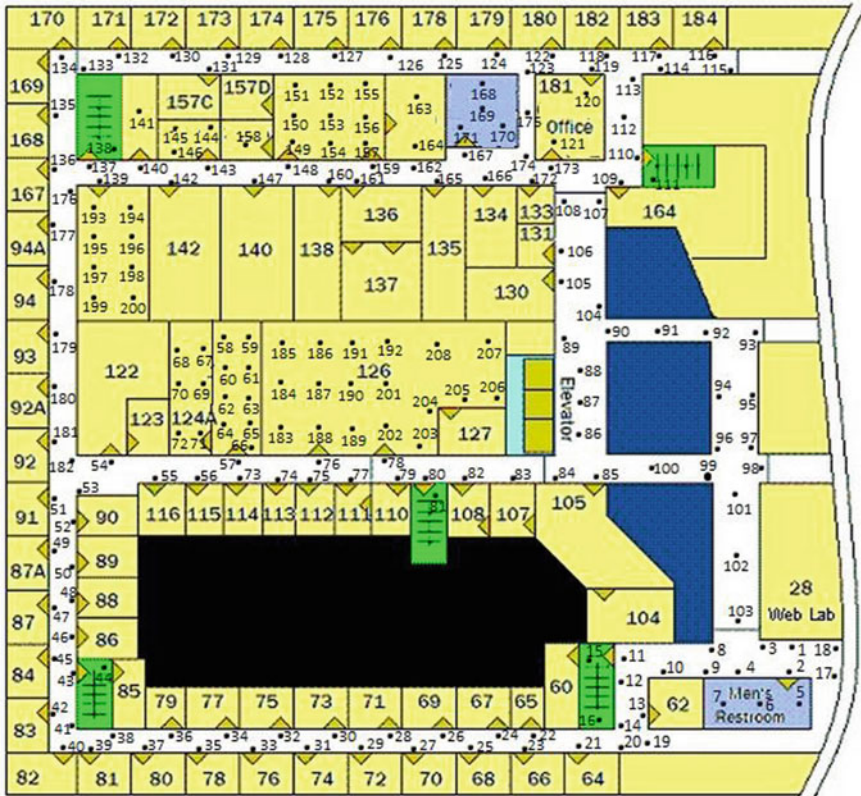
Fig. 1 Example of surveyed area: Wi-Fi RSSI fingerprint data were obtained at 208 sample locations (shown as dots) on the computer science department floor (68 m × 63 m) at UMass Boston. There are in total 138 Wi-Fi access points, and from those unreachable, the corresponding RSSI is set to -100 db. At each sample location, the corresponding fingerprint is the average of the RSSIs observed at this location. RSSI was measured by a person carrying an Android phone in no particular heading direction
