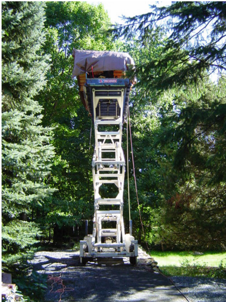
Fig. 1 This figure shows the lift with the experiment. The antennas are at the far end of the lift from the viewer under the roof that was built to shield the equipment from the elements. This picture was taken in September with the foliage largely still present. The cables coming from the lift are a ground cable to an earth ground and one of four tethers used in windy conditions
