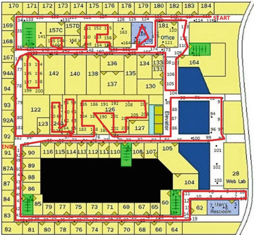
Fig. 5 A test trajectory visiting 185 locations on the computer science department floor (68 m × 63 m) at UMass Boston
