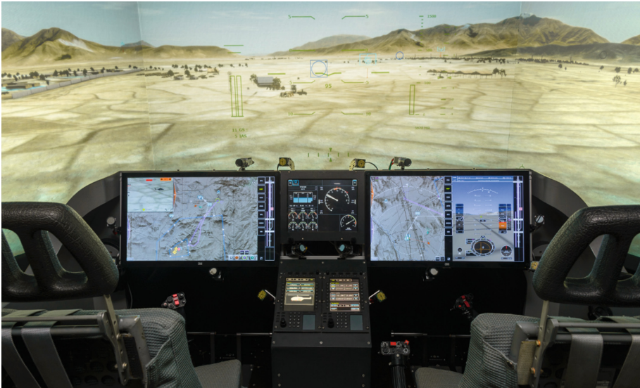
Fig. 4. Helicopter mission simulator at the IFS
