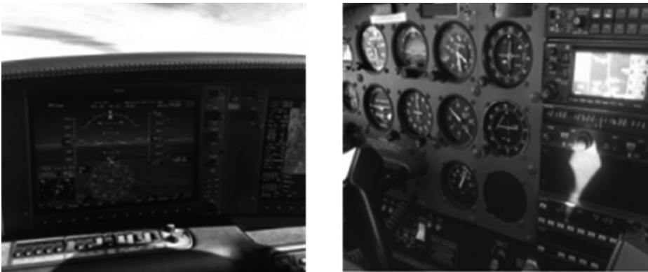
Fig. 4. Glass cockpit display (left) and traditional analogue display (right)
