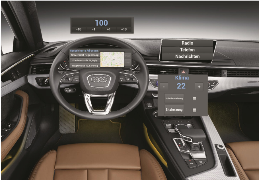
Fig. 2. Display setup in the prototype with speed control, navigation system, infotainment system and climate control. (Color figure online)
