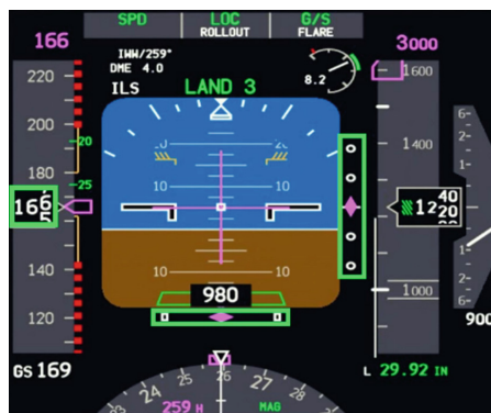
Fig. 2. Proposed modified flight mode annunciator by green color border (Color figure online)
