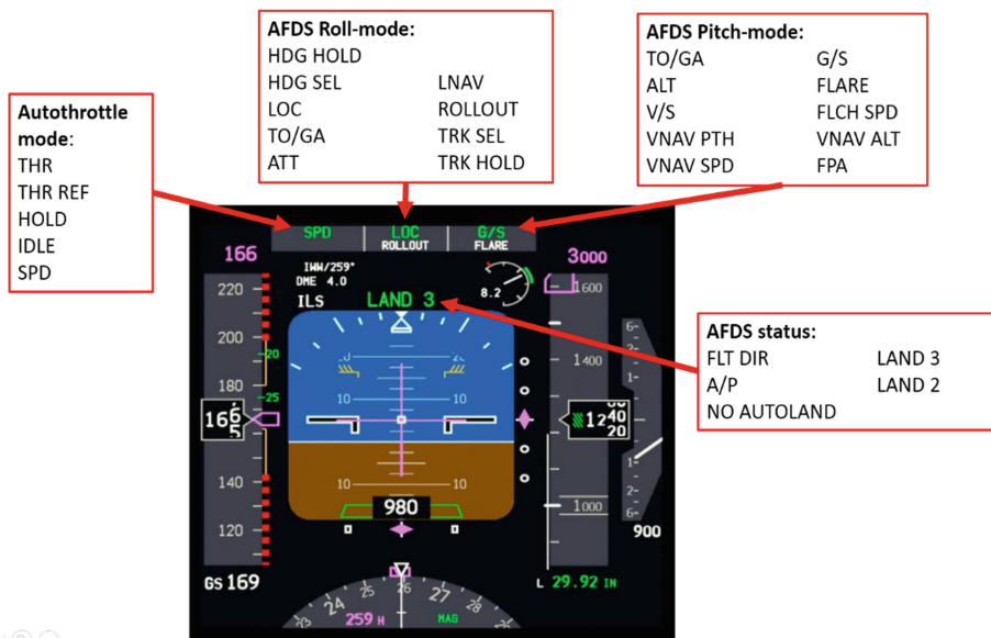
Fig. 1. Complex nature of flight mode annunciation in current display style (Color figure online)
