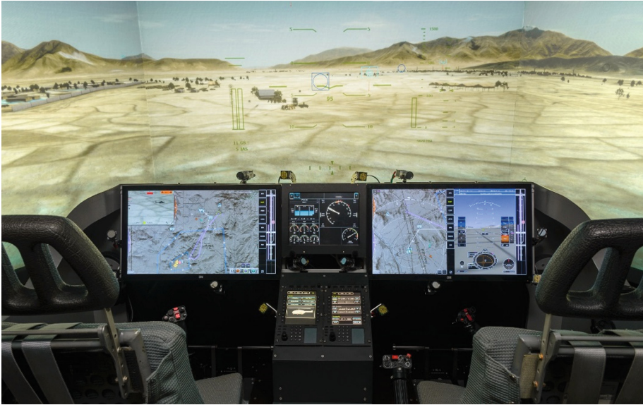
Fig. 11. Helicopter mission simulator at the Institute of Flight Systems, which we use to implement and evaluate the associate system for MUM-T missions.
