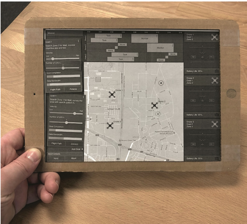
Fig. 2. Early paper prototype of a swarm interface. This version has more controls which we later removed like velocity and drone allocation sliders.
