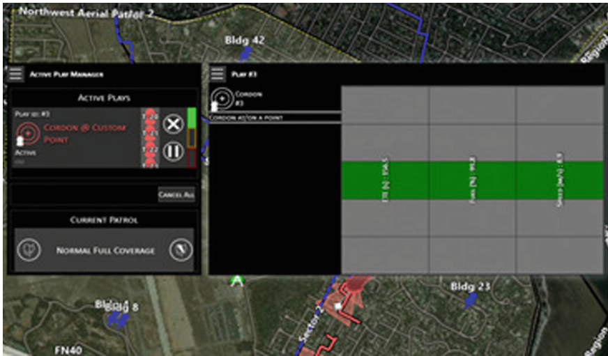
Fig. 3. The Plan Monitor displays plan health for active plays based on several criteria such as vehicle energy and time to destination.
