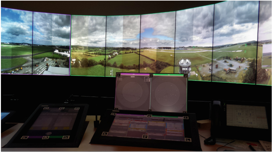
Fig. 1. The Module of multiple remote tower control system comprised by Electronic Flight Strip (EFS), Out of the Window (OTW), Radar Data Processing (RDP), Information Data Processing (IDP) and Voice Communication System
