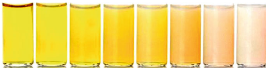
Fig. 16.5 Color dependence on the size of silver nanoparticles (size increases from left to right)
