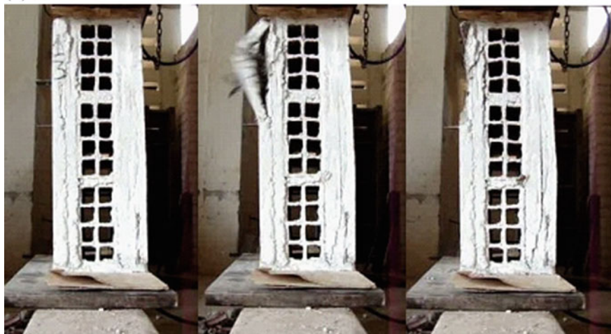
Fig. 14 Rupture of the a 2 block prisms and b 3 block prisms with a coating of 3.0 cm and a mix ratio of 1:1:6 reinforced with a POP mesh of 10 \times 10 cm and 4.2 mm of diameter
