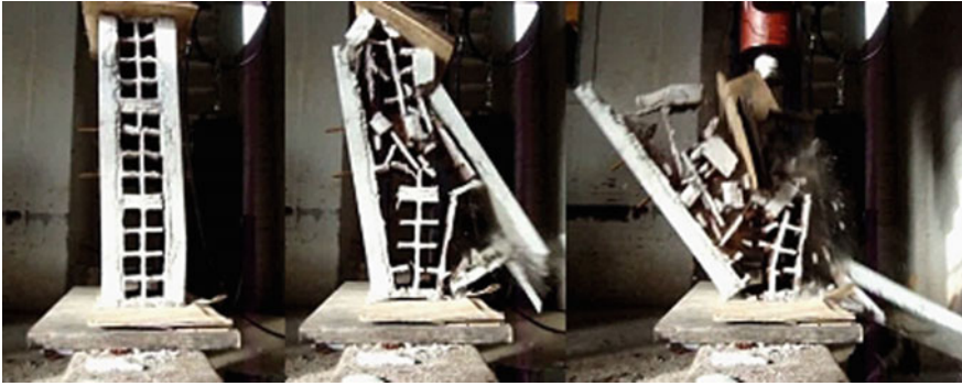
Fig. 15 Rupture of the 3 block prisms with a coating of 3.0 cm and a mix ratio of 1:0.5:4.5
