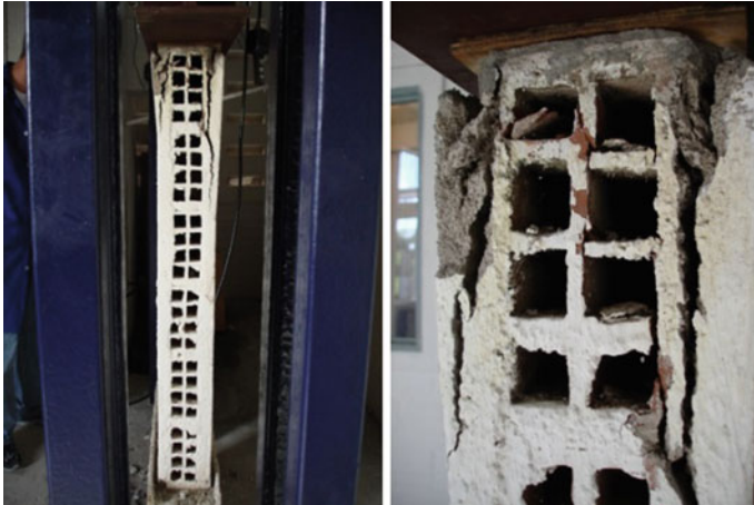
Fig. 16 Rupture mode of coated wallet specimens
