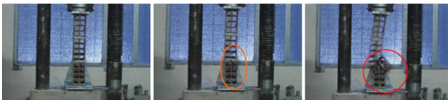
Fig. 7 Prisms of uncoated ceramic blocks: evolution of rupture
