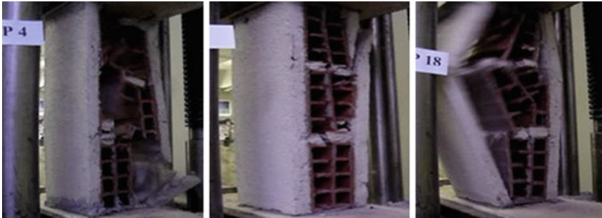
Fig. 9 Ceramic block prisms with coating and steel mesh
