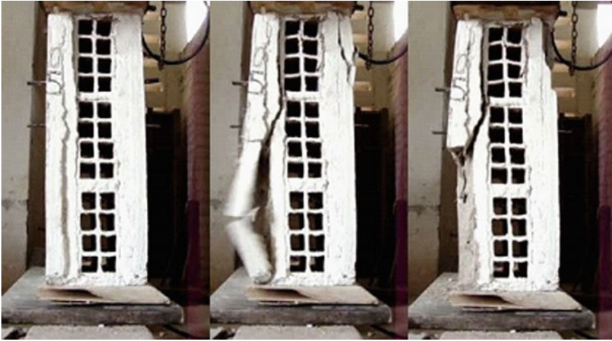
Fig. 17 Rupture of the 3 block prisms with a coating of 3 cm and a mix ratio of 1:1:6 reinforced with a POP mesh of 10 × 10 cm and 4.2 mm of diameter
