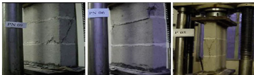
Fig. 11 Rupture of uncoated concrete block prisms
