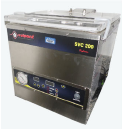
Fig. 13 a Device used for vacuum storage. b Samples of banana stored under vacuum
