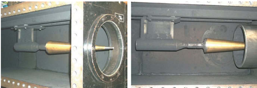
Fig. 1 Blunt cone model in the test section with nozzle removed and with nozzle in position before a shot. Note that the nozzle recoils by up to 120 mm during a shot
