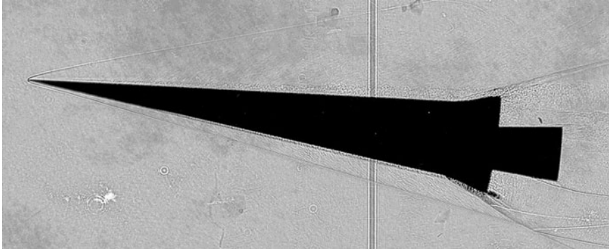
Fig. 3 The shadowgraph image of test ZL-13 ( Ma = 5.77 , Re/L = 8.56 \times 10^7 \text{ m}^{-1} , \alpha = 7.9^\circ )
