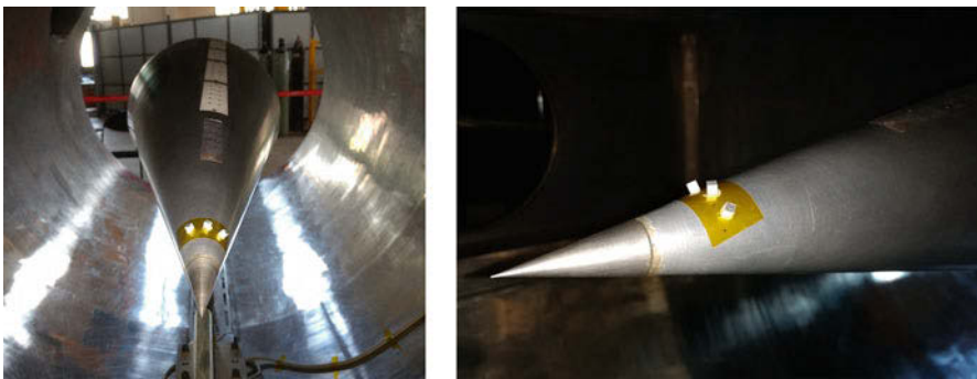
Fig. 2 800-mm-long cone model with MACOR inserts housing thin-film sensors (left) and a close-up of the trips (right)
