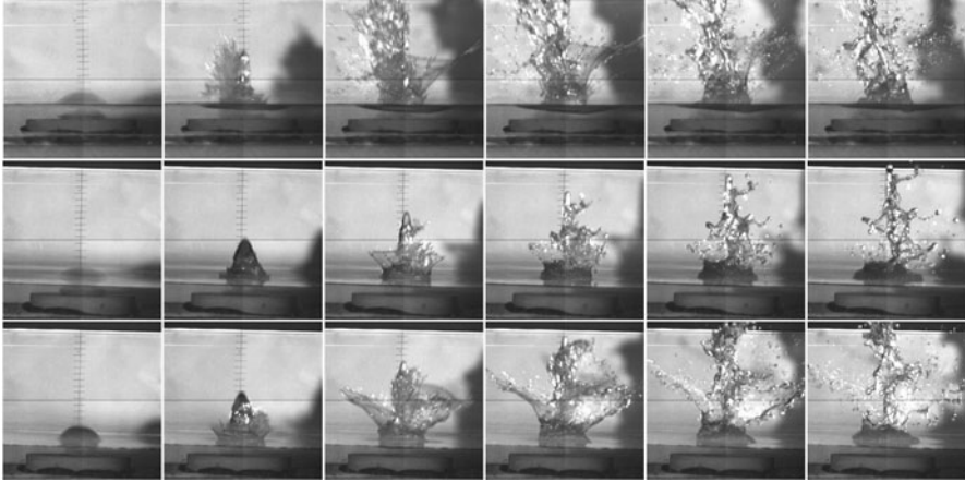
Fig. 7 Jets from the spherical, parabolic, and plane disks, with a driver pressure of 4 bar, 45 mm water depth. 20 ms between frames
