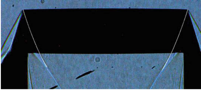
Fig. 5 Overlaid experimental and empirical results where R_c = 2 , L_w = 0.5 and \alpha = 4^\circ at Mach 3.6
