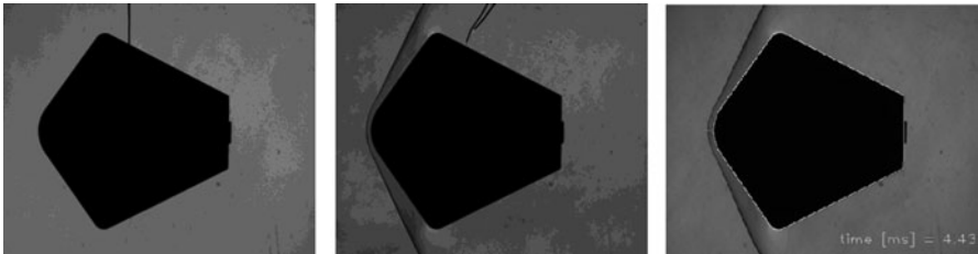
Fig. 3 Visualization of a capsule model prior to the run, at detachment from the threads and during the free-flight phase within the test time window (from left to right). The white line on the outer contour shows the detected geometry and the white line at the stagnation point the interrogation zone for the shock stand-off distance detection
