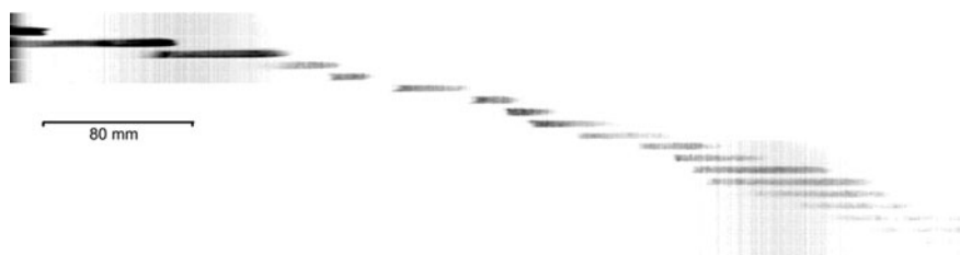
Fig. 2 Serial frames of the flame front and combustion products for acetylene-air mixture ( ER = 1.4 ) in inverted colors after entry into the narrow channel. Time interval between frames is 80 \mu s
