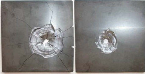
Fig. 1 Rear-side views of bulk (left) and layered (right) ceramic plates impacted under a similar condition [2]
