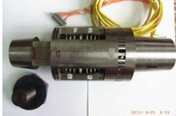
Fig. 3 The six-component strain balance designed for JF12 shock tunnel
