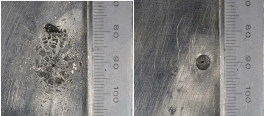
Fig. 3 Pictures of craters initiated on Al-plate for (left) dense-2 and (right) porous-2
