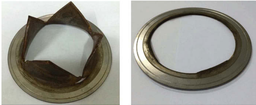
Fig. 2 Diaphragms in experiments, with the left in backward driving and the right forward
