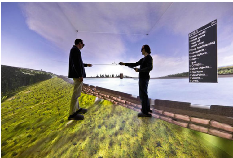
Fig. 5.3 The Cave Automatic Virtual Environment (CAVE). The CAVE gives researchers a fully immerse, 3-D simulation environment to analyze and discuss their computations. Created by the department of visualization at the high-performance computing center Stuttgart (HLRS), University of Stuttgart. Courtesy of the HLRS, University of Stuttgart
