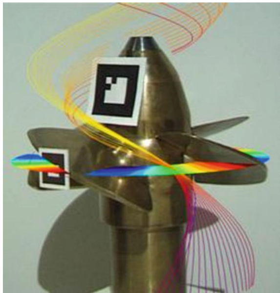
Fig. 5.4 Water flow is simulated interactively and displayed on top of a Kaplan turbine. Created by the department of visualization at the high-performance computing center Stuttgart (HLRS), University of Stuttgart. Courtesy of Stellba Hydro GmbH & Co KG
