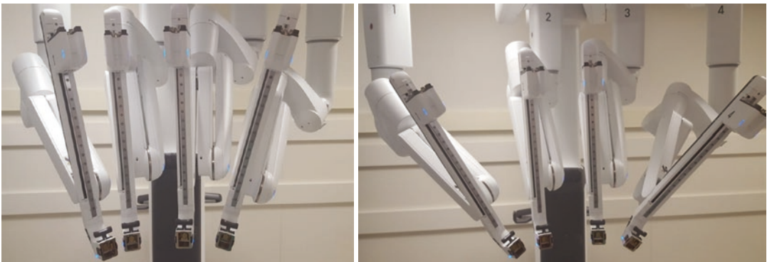
Fig. 8.5 Rotating the arms outward (at approximately 45° angles) creates greater distance at the elbows which reduces the likelihood of collision as the case progresses
