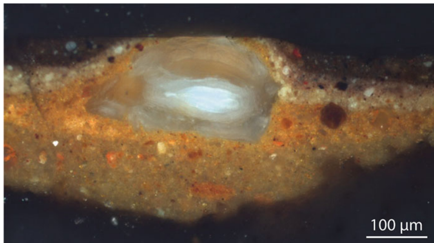
Fig. 3.1 Dark-field cross-polarized microscopy image of a large inclusion formed in the orange ground identified as lead soap in a paint cross-section from the painting Let the Children Come to Me by Jan de Bray (1663, Frans Halsmuseum). (Picture by L. Abraham)
