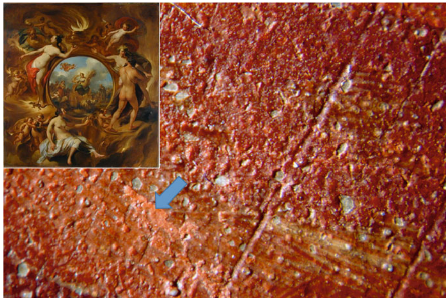
Fig. 1.7 Nicolaes Berchem (1620–1683), Allegory of Summer , c.1680, canvas, 94 × 88 cm, Mauritshuis, inv. 1091. Here lead soap aggregates, 100–200 \mu\text{m} in diameter, have broken through two layers of modern overpaint (indicated by arrow), causing masses of pinpoint paint losses. Overall (insert) and microscope detail from red drapery of standing figure left of center (Noble et al. 2005)
