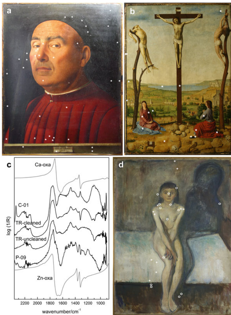
Fig. 10.2 Three case studies showing the presence of metal oxalate patinas: two ancient paintings (a) Trivulzio's portrait (1476) (Bellucci et al. 2010) and (b) The Crucifixion (1475) by Antonello da Messina and one modern painting (d) Puberty (1894) by Edvard Munch (Rosi et al. 2015). (c) Reflection mode FTIR spectra (black lines) compared with reference standards of zinc and monohydrated calcium oxalates (grey lines); spectra TR-uncleaned and TR-cleaned recorded on painting (a) and spectrum C-01 recorded on painting (b) showing example measurements for the identification of hydrated calcium oxalate on the points marked with asterisks in (a) and (b). Spectrum P-09 is representative of the measurements on painting (d) where zinc oxalate has been specifically identified on the measurements points marked with white pluses. On painting (d) white circles indicate areas where the acquired spectra show the presence of small amount of oxalates without providing for metal speciation
