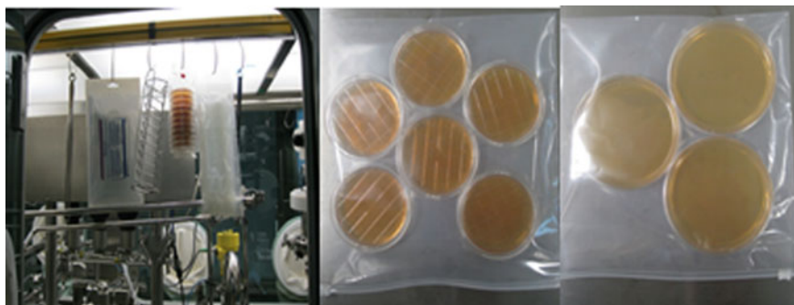
Fig. 21.7 Zipper bags firmly holding together the microbial plates while removal through RTPs; equipment located at F. Hoffmann-La Roche, Basel, Switzerland
