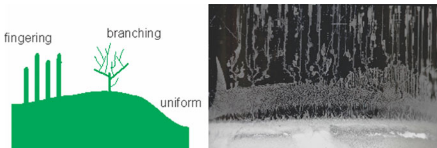
Fig. 14.3 Marangoni flow patterns and example of the resulting “fogging” on a lyophilized product vial
