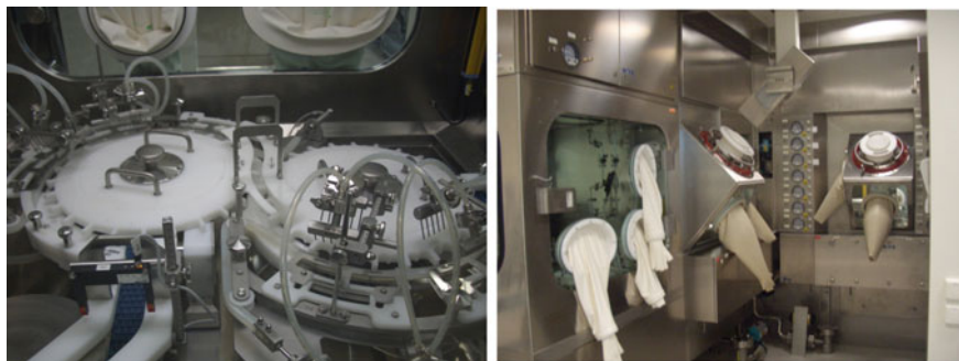
Fig. 21.4 Validated outside washing of vials after crimping in the containment, drying of the vials without heat-exposition; equipment located at F. Hoffmann-La Roche, Basel, Switzerland
