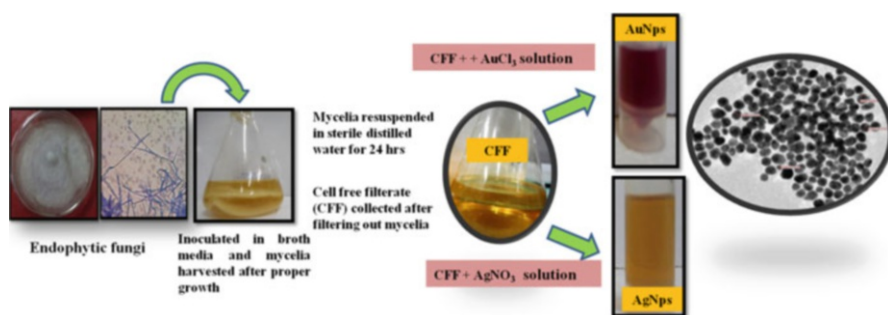
Fig. 17 Endophytic fungi mediated synthesis of gold and silver nanoparticles
