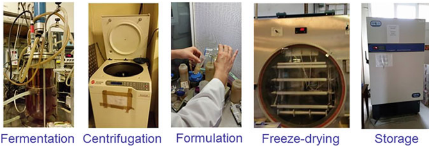
Fig. 22.9 Steps of the freeze-drying process. Control parameters at every point in the process chain can influence the quality of bacterial starters
