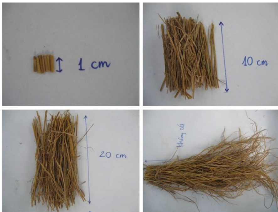
Fig. 9.2 Different sizes of rice straw cut for the testing: 1 cm, 10 cm, 20 cm, and uncut straw
