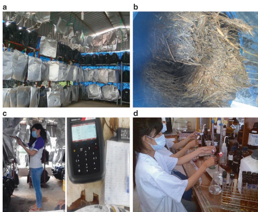
Fig. 9.4 Experimental setup and sampling activities. (a) Digesters with different treatments. (b) Rice straw after 60 fermentation days. (c) Recording operating units and gas components. (d) Sample analysis in the lab
