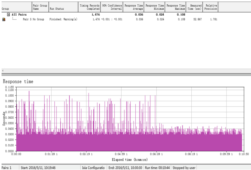
Fig. 13. Round trip latency value in network B
