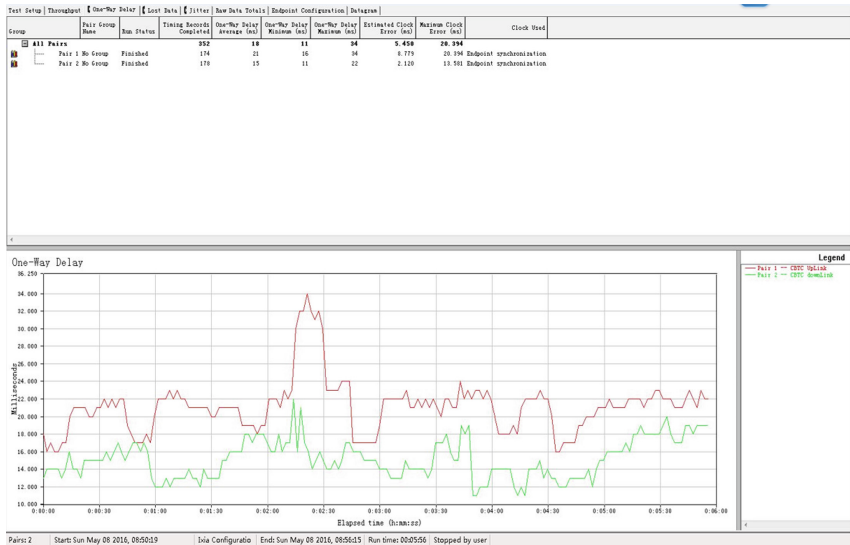
Fig. 14. Handover-latency example in network A
